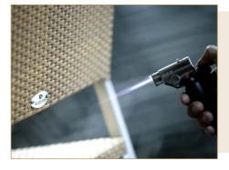
Scratch marks or abrasion to the edges of the fibre can be repaired by very briefly and carefully applying heat (i.e. the flame of a cigarette lighter) to the affected area and rubbing along the length of the fibre with a piece of hard cardboard to restore a smooth edge. Even if fibres are accidentally cut or broken, a piece of furniture can generally be repaired successfully.
