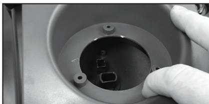
Step 3 - Lift off the blue filter casing.
