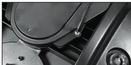
Step 4 - Undo the screws on the lid of the UV compartment.
