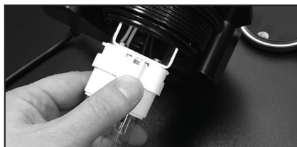
Step 8 - Unclip the bulb and replace. CAUTION: NEVER LOOK AT A LIT UV BULB.
